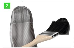
Apply a thin film of contact adhesive, suitable for TPU material. Then, leave to air dry.
